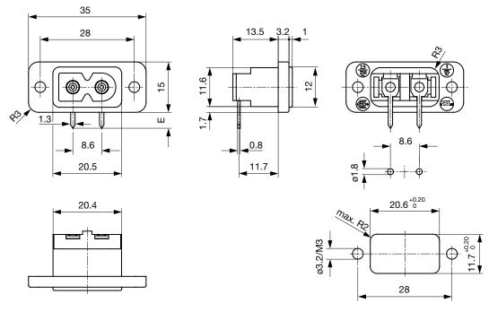
E: PCB terminal standard: 4.8 mm E: PCB terminal short: 3.2 mm
