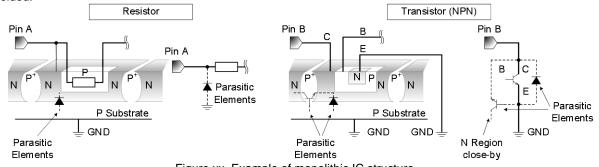
Figure xx. Example of monolithic IC structure
