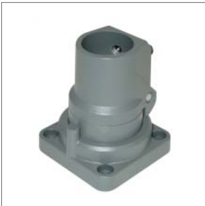
Foot stand, swivelling Cast aluminium with steel inner tube and flange mounting. Swivelling range 250° (cannot be limited or stopped)
