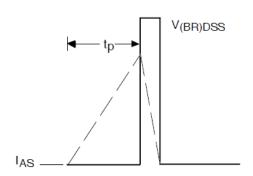
Fig 22b. Unclamped Inductive Waveforms
