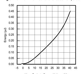
V<sub>DS,</sub> Drain-to-Source Voltage (V) **Fig 11.** Typical Coss Stored Energy
