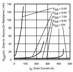
Fig 12. Typical On-Resistance vs. Drain Current
