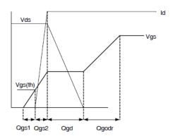
Fig 24b. Gate Charge Waveform
