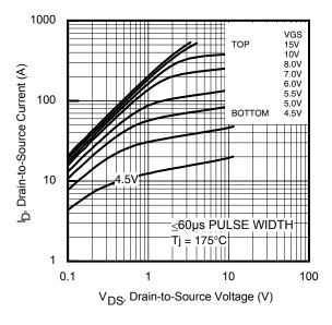
Fig. 2 Typical Output Characteristics
