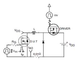
Fig 22a. Unclamped Inductive Test Circuit
