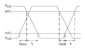
Fig 23b. Switching Time Waveforms
