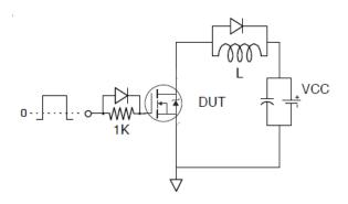
Fig 24a. Gate Charge Test Circuit
