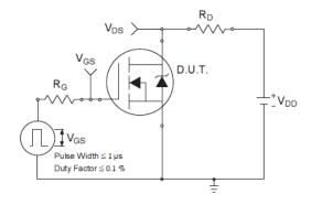
Fig 23a. Switching Time Test Circuit
