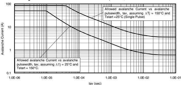
Fig 14. Typical Avalanche Current vs. Pulsewidth
