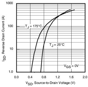
Fig. 7 Typical Source-to-Drain Diode Forward Voltage
