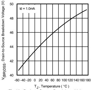
Fig 10. Drain-to-Source Breakdown Voltage
