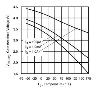
Fig 17. Threshold Voltage vs. Temperature
