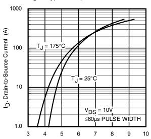
V<sub>GS</sub>, Gate-to-Source Voltage (V) **Fig. 3** Typical Transfer Characteristics
