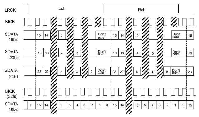
Figure 16. Mode 3 Timing (LRP = BCKP bits = "0")
