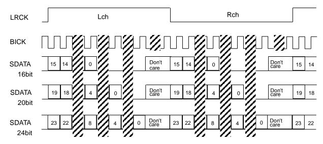
Figure 15. Mode 2 Timing (LRP = BCKP bits = "0")
