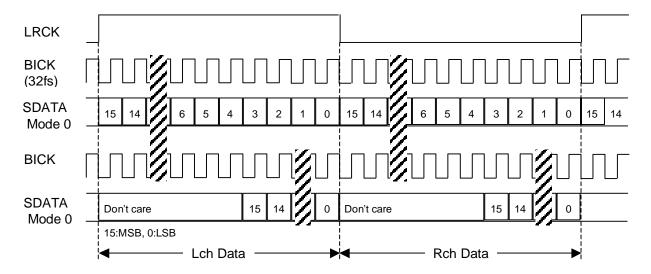
Figure 13. Mode 0 Timing (LRP = BCKP bits = "0")
