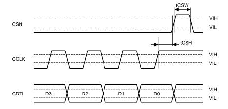
Figure 8. WRITE Data Input Timing
