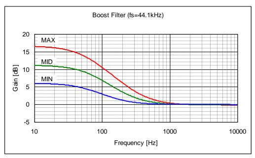
Figure 2. Boost Frequency (fs=44.1kHz)
