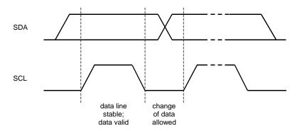
Figure 37. Bit Transfer on the I<sup>2</sup>C-Bus
