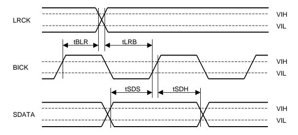
Figure 5. Serial Interface Timing (Slave Mode)
