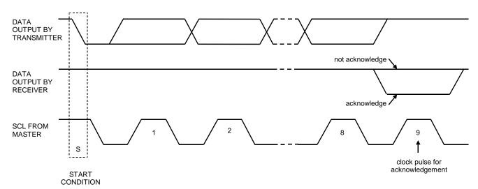
Figure 36. Acknowledge on the I<sup>2</sup>C-Bus
