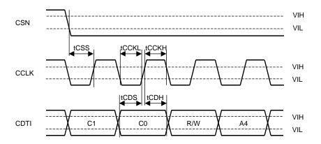
Figure 7. WRITE Command Input Timing
