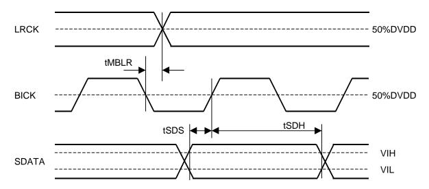
Figure 6. Serial Interface Timing (Master mode)
