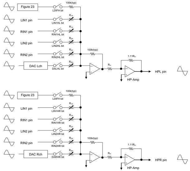
Figure 21. Summation circuit for HPL/R output
