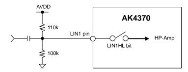
Note: If the path is OFF and the signal is input to the input pin, the input pin should be biased to a voltage equivalent to VCOM voltage (=  $0.475 \times AVDD$ ) externally.
