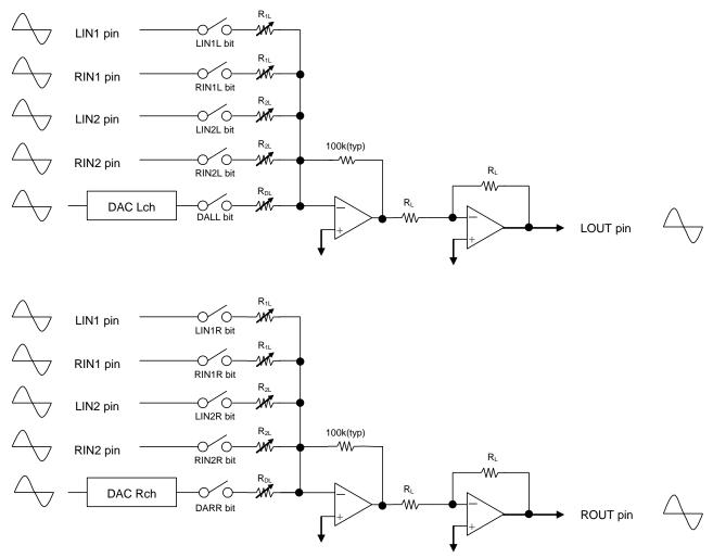
Figure 22. Summation circuit for stereo line output
