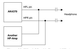
Figure 20. Wired OR with External HP-Amp
