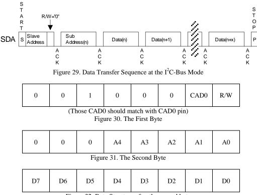
Figure 32. Byte Structure after the second byte
