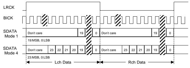
Figure 14. Mode 1, 4 Timing (LRP = BCKP bits = "0")
