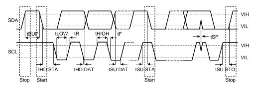
Figure 9. I<sup>2</sup>C Bus Mode Timing
