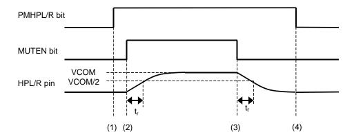
Figure 18. Power-up/Power-down Timing for the Headphone-Amp
