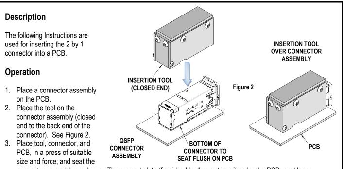
connector assembly as shown. The support plate (furnished by the customer) under the PCB must have clearance for the connector pins as they pass through the PCB.
