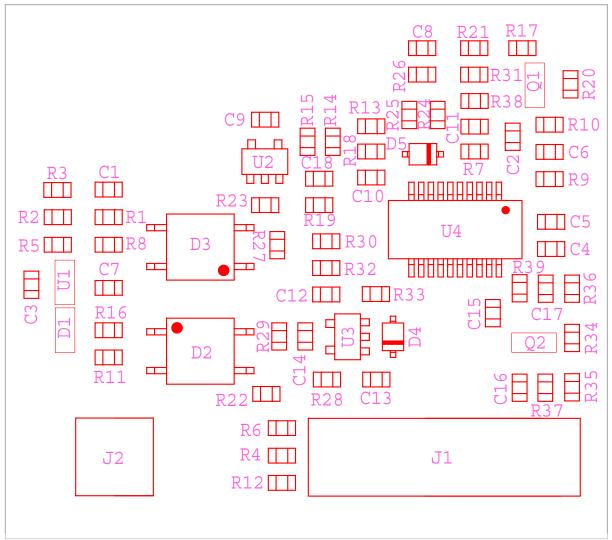
FIGURE 5. ISL6754 CONTROL CARD TOP ASSEMBLY
