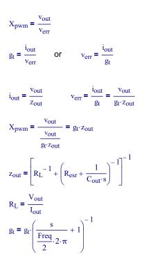
This gain function is used in the bode analysis for the ISL6752 and ISL6754.
