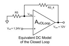
Because the Xtotal.gain includes the degenerative gain of the voltage scaling resistors R3\_4 and R5, we must exclude this gain stage from this load regulation analysis.
