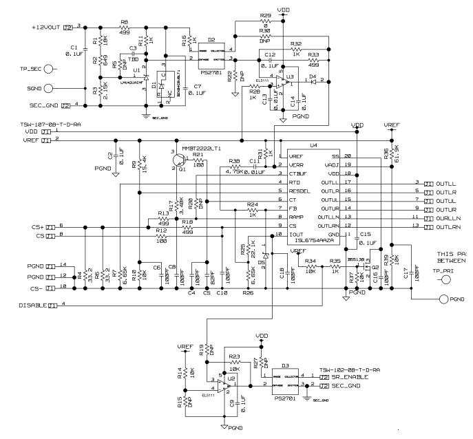
FIGURE 3. ISL6754 CONTROL CARD SCHEMATIC
