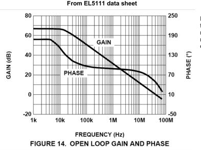
Note that the phase of this graph is the output referenced to the negative input of the opamp.
