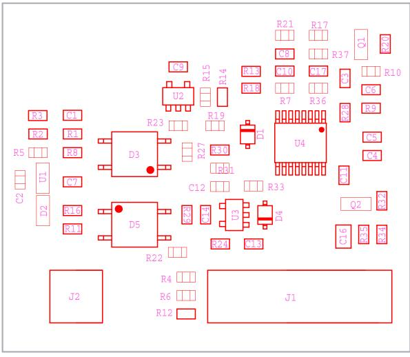
FIGURE 8. ISL6752 CONTROL CARD TOP ASSEMBLY
