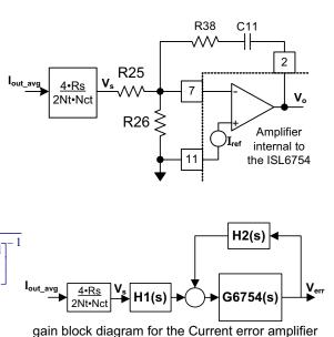
These values are used to compensate the current regulation closed loop.
