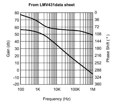
The open loop transfer function of the LMV431 is created here by inserting poles as necessary to recreate the Gain/Phase plot found in the data sheet. Note that the phase shift is relative to the input.
